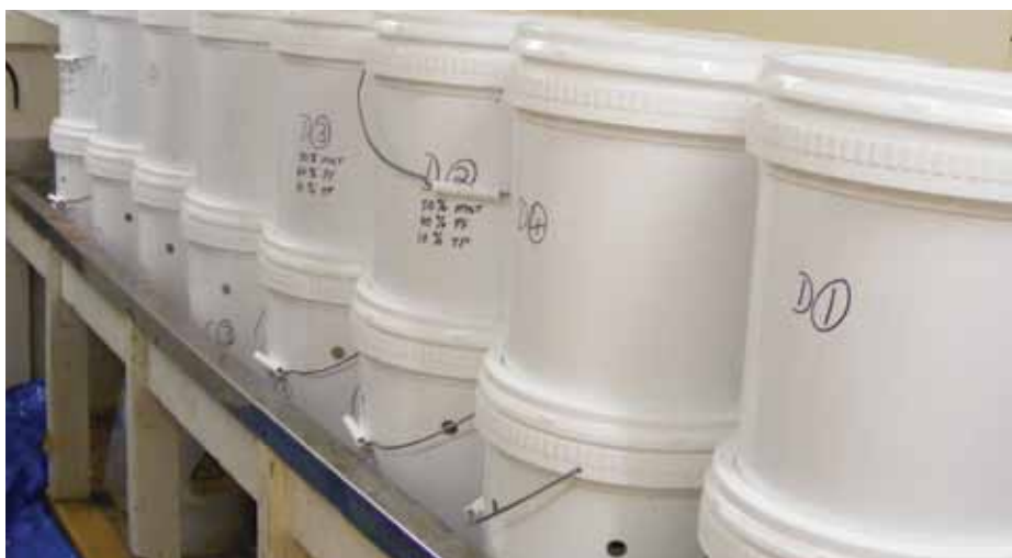
The final set up comprised of 16 vermi-composting containers. The bucket on top contains the worms and the compost mix in aerated conditions, whilst the bucket below contains a funnel and glass bottle that is designed to collect worm leachate for analysis.
